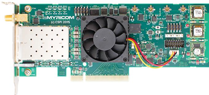
**C-Class** – This is our cost-optimized series. It is 10 Gbit only and comes in one or two port versions. There are several form factors including: PCIe low profile, IBM BladeCenter, and an industrial/defense optimized PC/104. The C-series supports both Windows and Linux.
