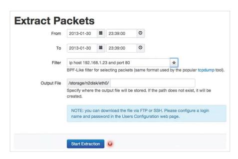
The nVoy UI allows simple and powerful specification of packets to be extracted based on capture time and or BPF-like filtering.
